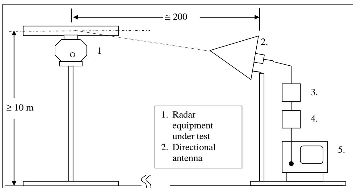
Figure D.2: Measurement of spurious emissions and out of band emissions,
