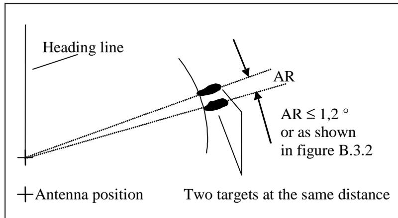
**Figure C.3: Definition of the Azimuthal Resolution (AR)**
