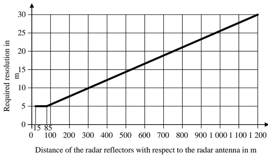
**Figure C.4: Azimuthal Resolution depending on the range**
